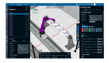
OCTOPUZ Offline Robot Programming (OLRP) software enables complex robot applications to be programmed in a virtual, offline environment, without disruption to your manufacturing process and without the need for an onsite programming expert. OCTOPUZ programs multiple robot brands, configurations, and applications together and outputs code for use in real-world industrial applications.
